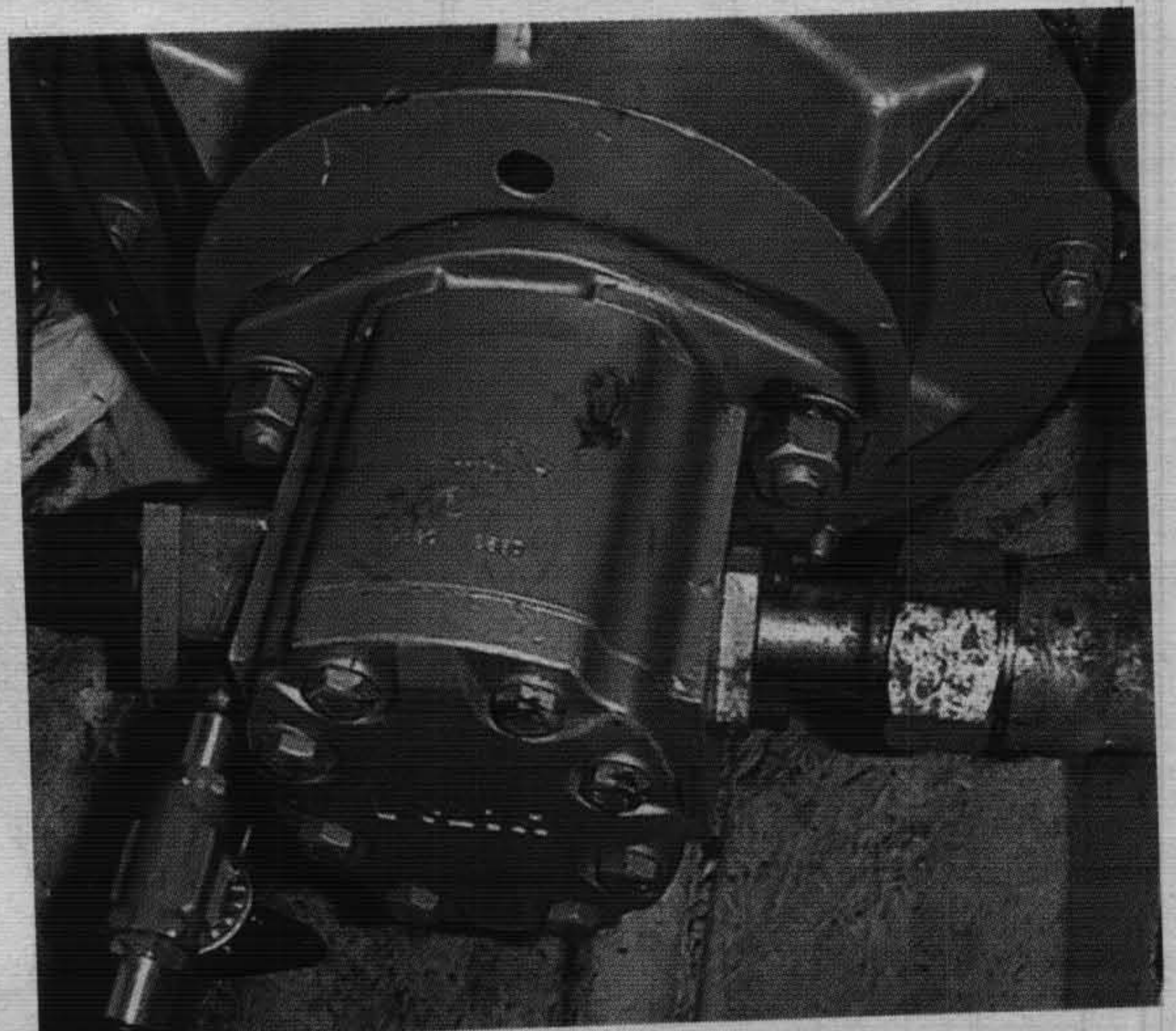
The Ultra gear pump yields 2100psi, but we had to modify the original mounting flange.
