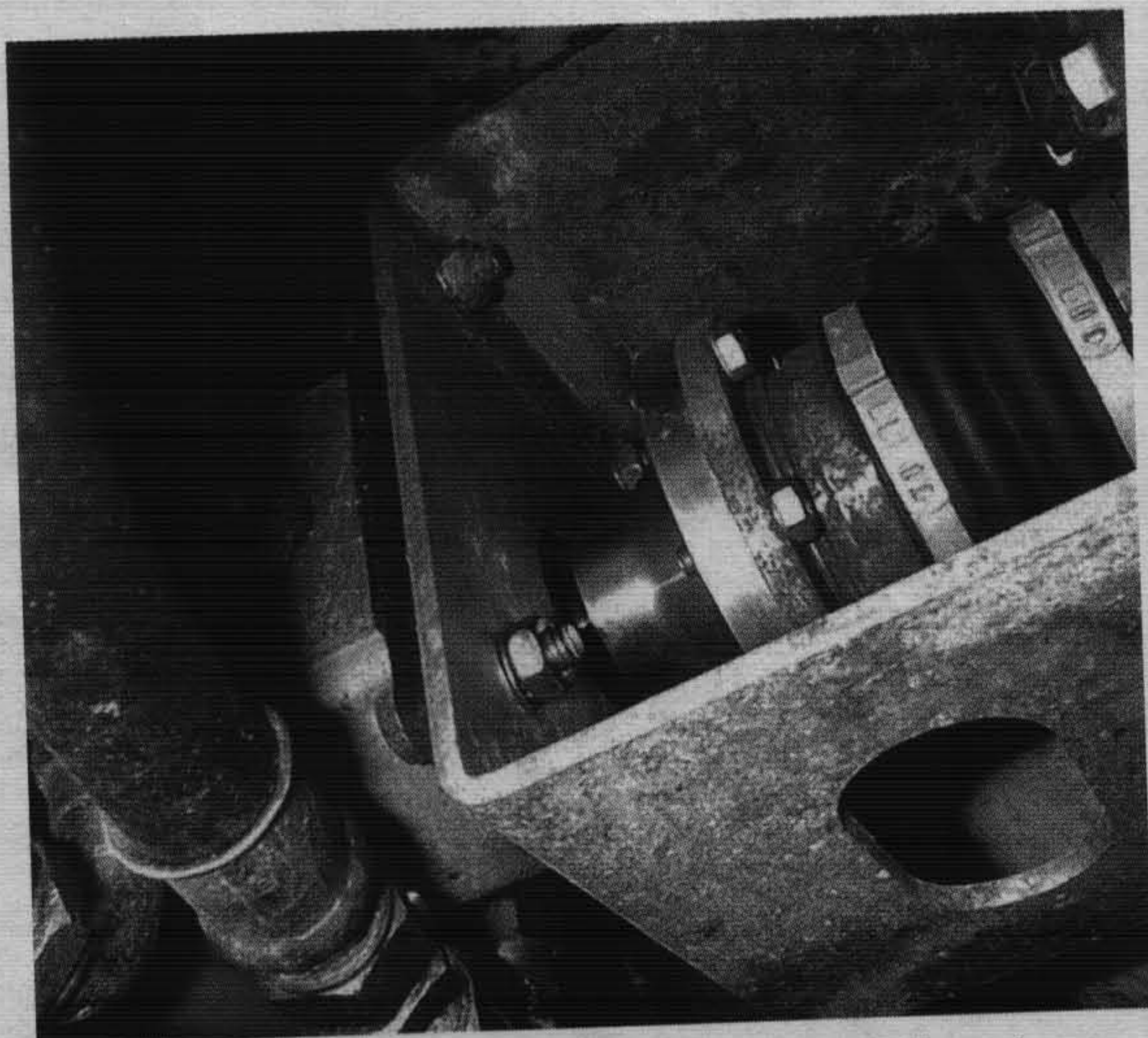
Because the Cassapa gear pump had no thrust bearing, we used an Aquadrive CV unit.
